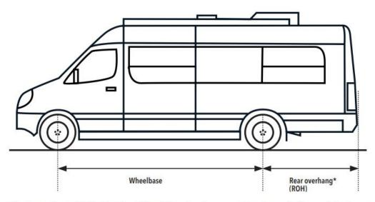
\*Rear overhang (ROH): Shall be 60% of the wheelbase or 3.7 metres, whichever is the lesser., measured from the rear overhang line.
