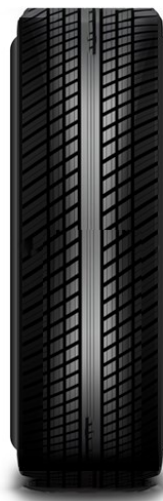
Thin tread along tyre edges
